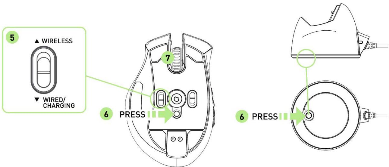
6. Press the pairing buttons on the Razer Naga Epic and Charging Dock. The lights on the Razer Naga Epic will start flashing to indicate the pairing process.
