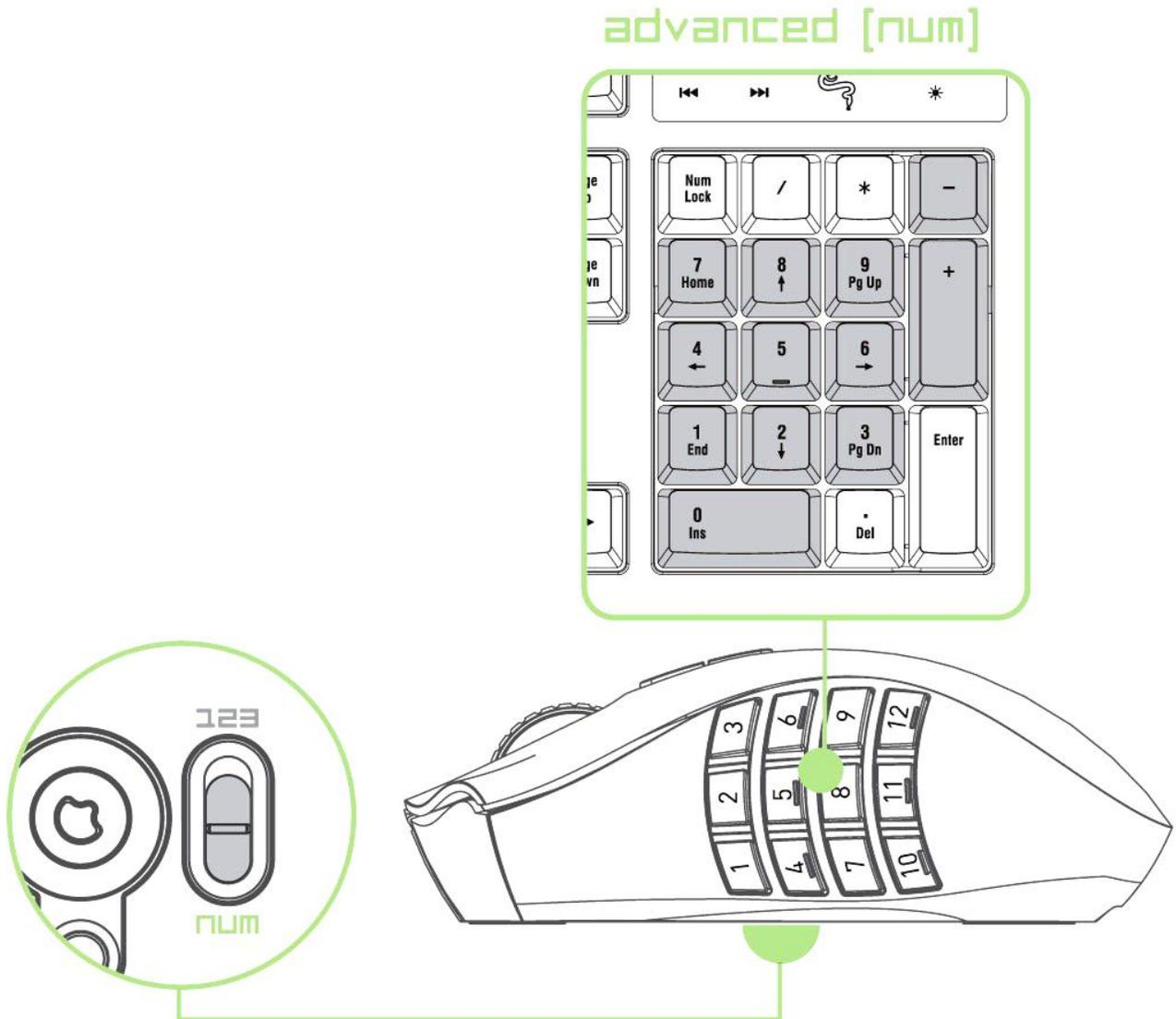
In the Advanced [Num] mode, the 12-button thumb grid works the same as a keypad's numerical keys. These buttons allow you to have quicker access to in-game commands without having the need to reach for the keypad.
