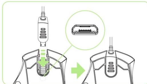
3. Plug mouse into the USB port of your computer. The Razer Naga Epic is then ready for use as a high performance wired mouse. In addition, its battery will start charging automatically in this wired mode.
