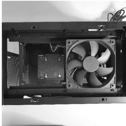
Up to two 120mm fans can be mounted at the bottom of the chassis' interior.
