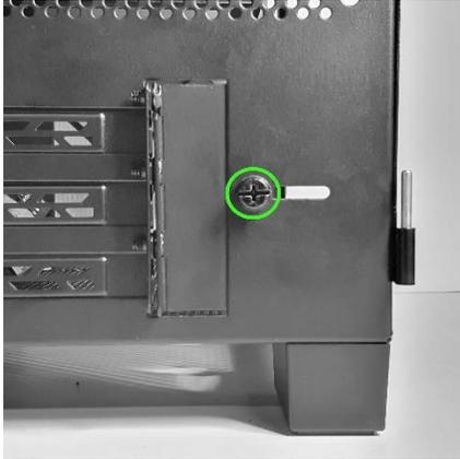
Slide the screw to the right to open the panel and then tighten the screw to keep it secure.
