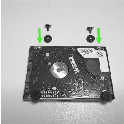
You can mount up to two 2.5" drives on the bottom interior of the chassis.
