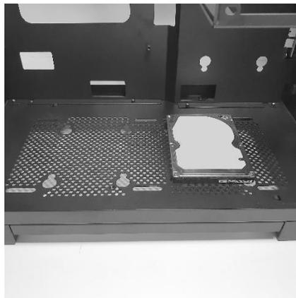
You can also mount a drive on the side exterior of the chassis.
