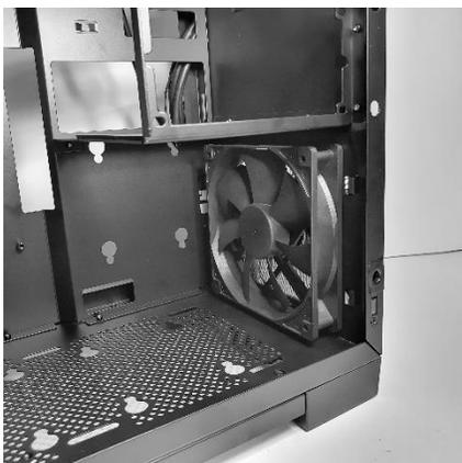
The back can accommodate up to a 120mm radiator and fan.
