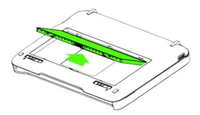
4. Press down the battery until the latches lock into place.
