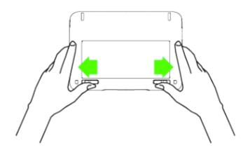
2. Remove the battery compartment door.
